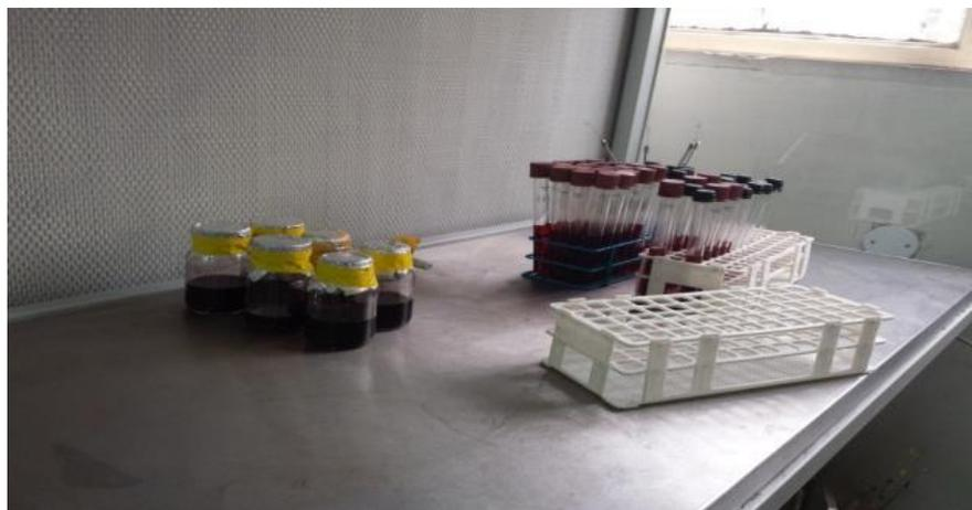
**Figure: 4. 7 Tanker Water Samples for Bacteriological and Physico-Chemical Water Quality Test**
