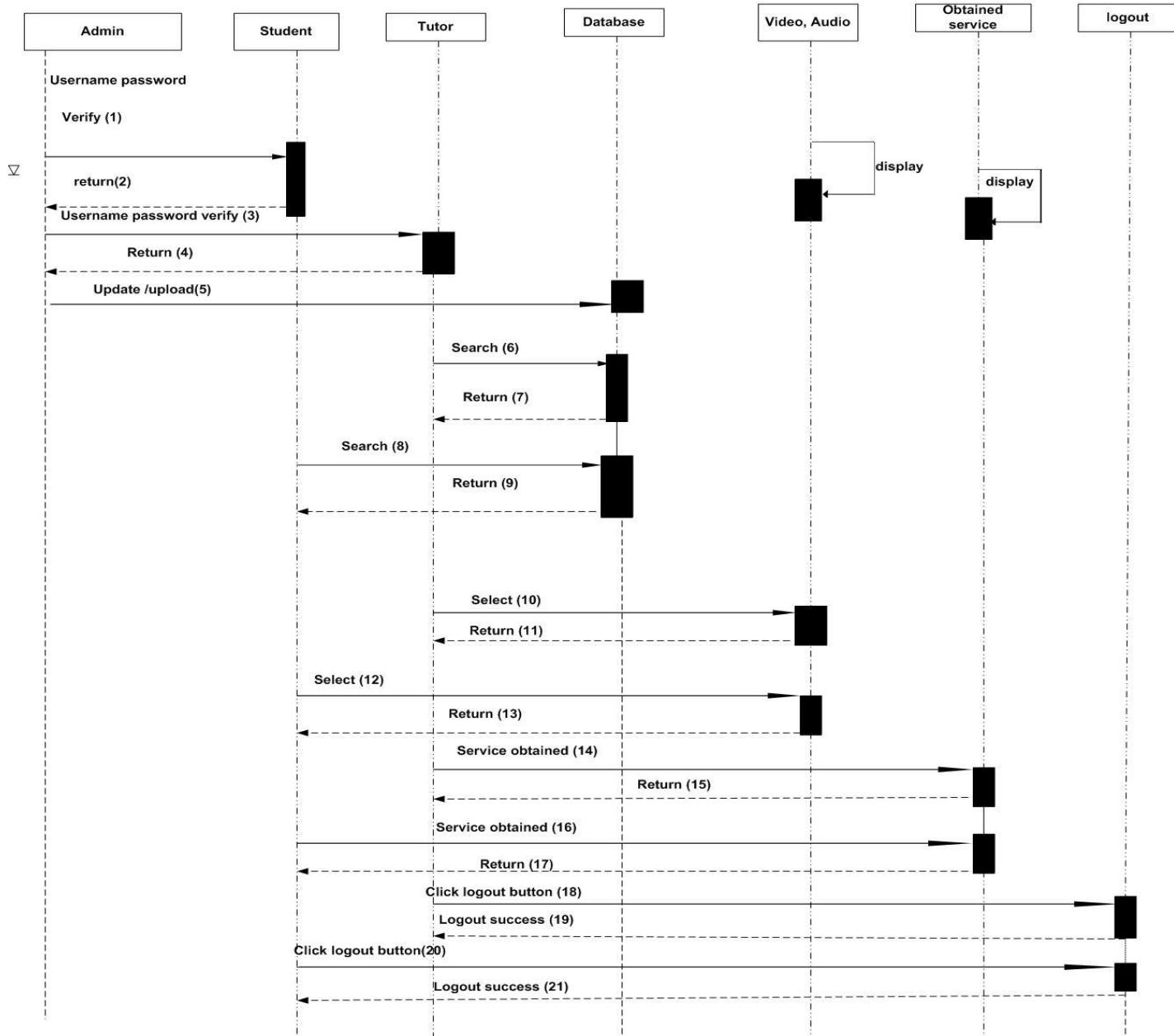
Figure 5.3: Sequence Activity flow for Mobile Based Tutoring
