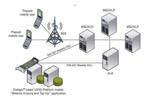
Fig.9. Components of USSD service [62]
