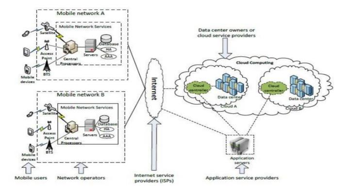
Figure: 2.1Architecture of Mobile Cloud Computing, Source: Dihn et al., 2011 [2011]
