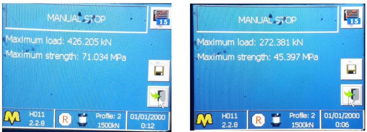
Figure 12 Result for compressive strength.
