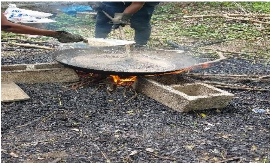
Figure 5 Melting plastic and mixing with sand
