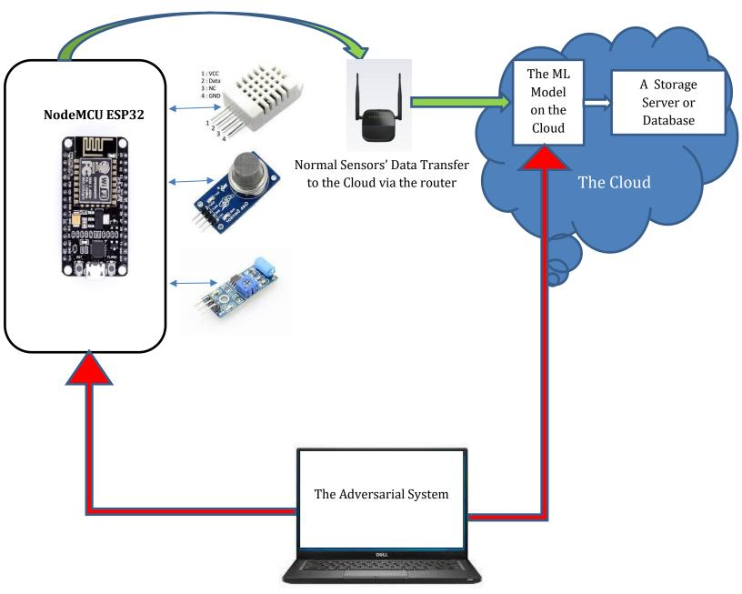
ARP poisoning, Sensors' data interception, and data modification performed by the Adversarial system prior to forwarding these modified Sensors' data to the cloud
