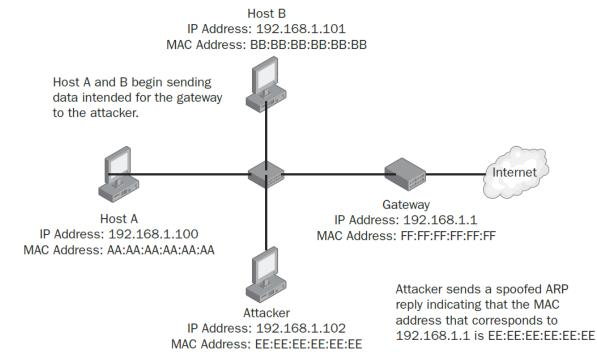
Figure 8: Example of MiTM attack using ARP Poisoning [19]
