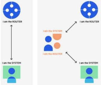
Figure 9: ARP Poisoning or ARP Spoofing [22]
