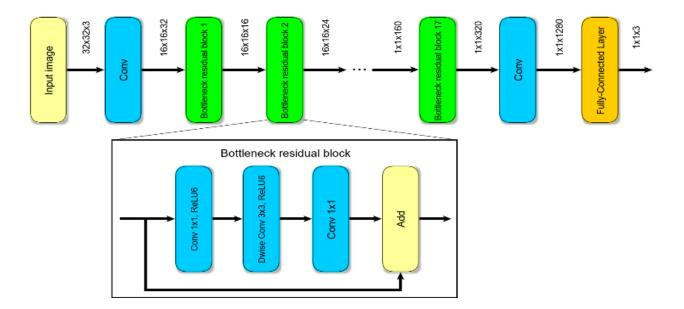
Figure 4-4. Architecture for MobileNetV2.
