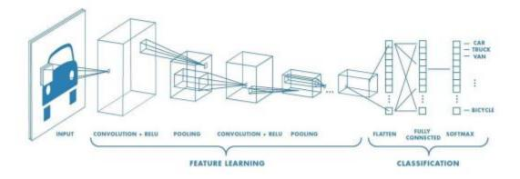
Figure 2-5. ConvNet Architecture [35].
